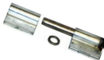
H412550LH BUTT HINGE, 4" L x 1 1/4" W, LEFT. FLUSH MNT WING STYLE, ZINC PLT STEEL, STAINLESS STEEL PIN 1/2" BUYERS
