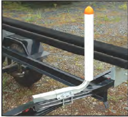
High Impact Pontoon Trailer Guide On's
